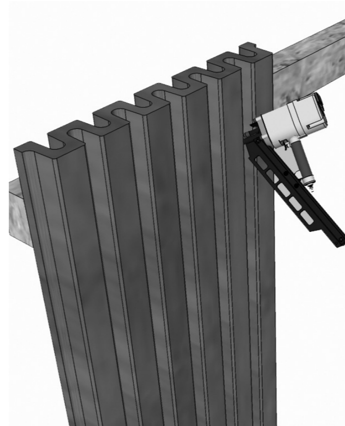
STEP 2 To make sure at least 2 nails fixed on the batten
